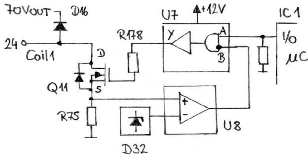
Note: The over current protection is disabled for all MOSFETs on current I/O-Boards by replacing all measuring resistors with 0 Ohm devices and additionally shorting them with a common wire. Obviously this circuitry caused problems, the additional wires could be a hint at some (unhealthy) oscillation tendency.
