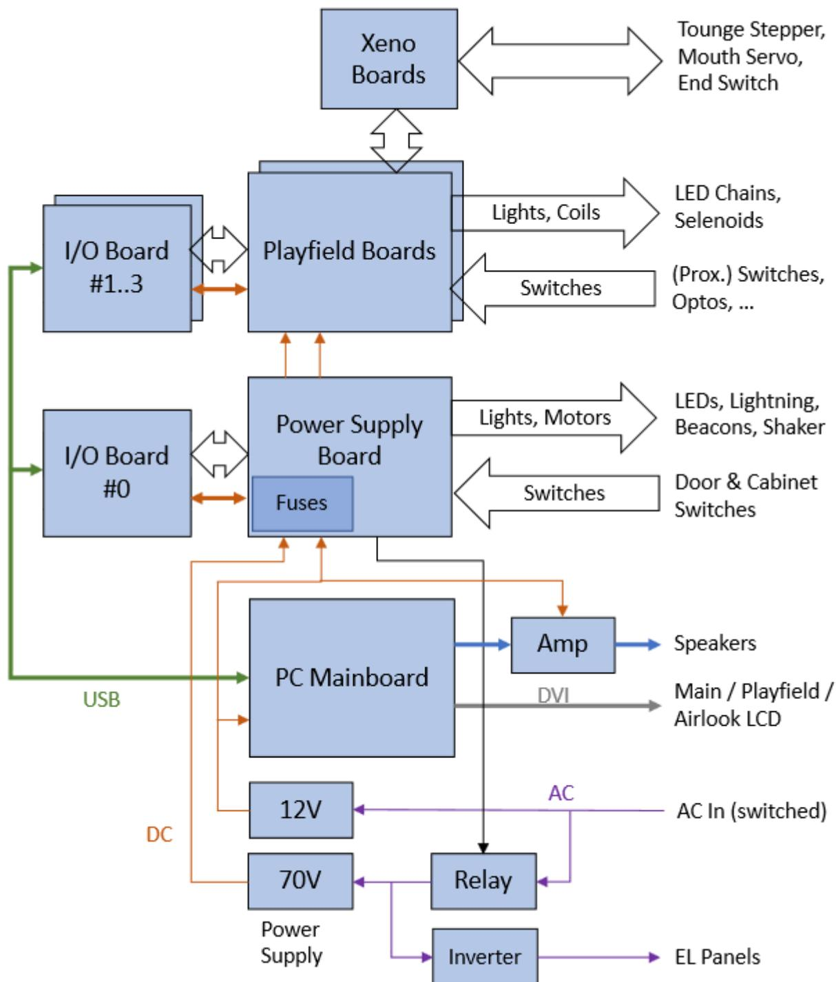
Unfortunately there are no schematics available for the I/O Board (as of Jan 2019) but it would be helpful to understand its functionality and circuitry for general maintenance as well as repair purposes. Therefore I inspected the boards for some time and here are my results.
