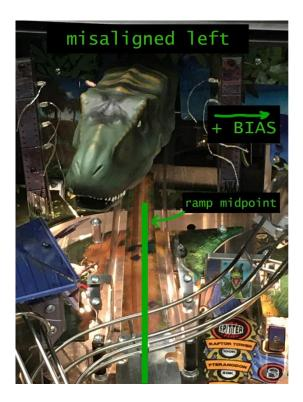
The following example is for a mis-aligned T-Rex that needs the **"T-REX STEPPER MIDDLE POSITION BIAS"** adjusted in the negative direction.
