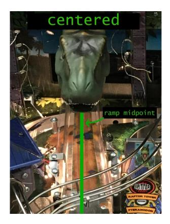
The following example is for a mis-aligned T-Rex that needs the **"T-REX STEPPER MIDDLE POSITION BIAS"** adjusted in the positive direction.
