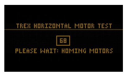
5) Once PLEASE WAIT: HOMING MOTORS is no longer visible observe the position of the T-Rex over the ramp. The T-Rex should be dead center above the ramp. If it strays to the left or right of the ramp there will need to be an adjustment made to the adjustment titled "T-REX STEPPER MIDDLE POSITION BIAS"
