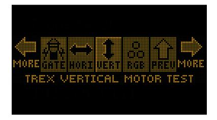
9) When the **T-REX VERTICAL MOTOR TEST** is running it will run a homing procedure just as the horizontal motor test did. Wait until **"Please Wait: HOMING MOTORS"** no longer appears.
