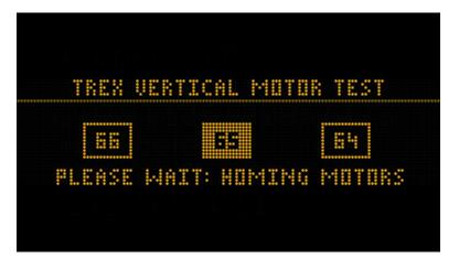
10) Press the "-" MINUS button to move the T-Rex head down to the Ramp.
