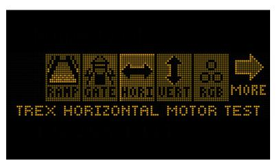
4) You should see the following message while the T-Rex performs the homing procedure. It will home the stepper motor and then perform a Left / Right / Center movement to recover any lost steps.
